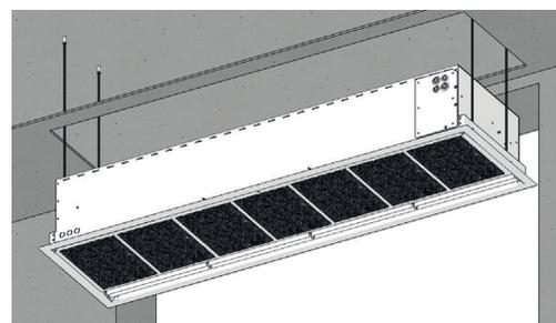
Due to the possibility of internal access to the suspension components, the door curtain can be additionally leveled after installation in the ceiling.
