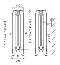
Manufacturing tolerance of ±2mm should be allowed in all dimensions.
