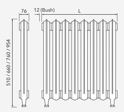
**Note** - When connecting bottom opposite ends 24mm must be added to 'L' dimension to allow for the reducing bushes. If connecting top/bottom same end then 12mm must be added to 'L' dimension plus valves.
